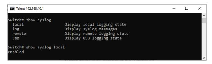
Here, you can see the sub fields of local, log, remote and usb are available. Adding one of these to the command, completes the command and executes.
